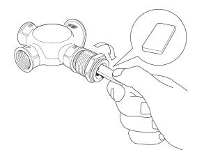
Once the orientation has been determined the straight connector which connects the Heatpump UFH kit to the manifold needs to be screwed into the return port. This is tightened using the straight connector tool supplied.
