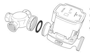
Connect the Heatpump UFH kit body to the pump using the pump nut which is pre-assembled ensuring the pump washer is inserted. Please take note of the directional arrow on the pump body.
