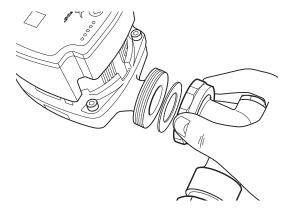
Connect the nickel plated elbow to the pump using the 1 ½" pump nut, ensuring the pump washer is inserted.
