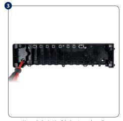
Mount the back side of the housing to the wall.
