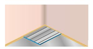
4. Start to lay the pipework into the preformed Foil Board using the HydroHeat CAD Design. Each insulation board will have pre-formed bend to allow for the return pipework.
